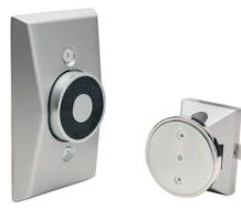
The LCN SEM7800 Series are heavy duty, electrically controlled door holding magnets. Magnets are fail safe and hold until the current is interrupted. A manual door closer is used to control and close the door. A choice of floor, recessed wall, or surface mounted wall magnets are available.
